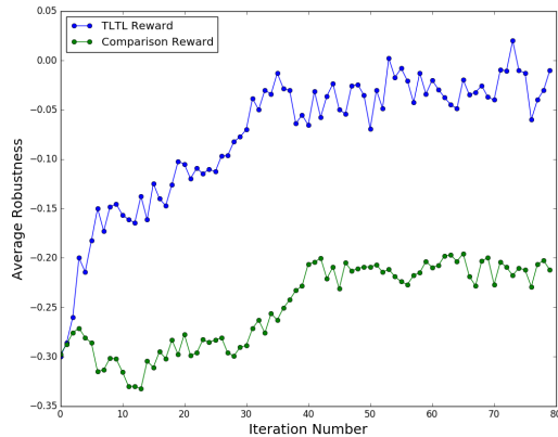
Fig. 4 : Training curves for Baxter toast-placing task. An episode is 100 time-steps long (around 6 seconds). Each update iteration uses 10 sample trajectories. Trained for 80 iterations
